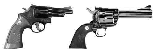
The two main types of revolvers. Left: Double-action revolver (Smith & Wesson Model 19). Right: Single-action revolver (Colt Single Action Army, colloquially known as the "Peacemaker"). An observer will note that on any single action, the trigger will be very close to the back of the trigger guard because the trigger pull need only release the already cocked hammer. On a double action, the trigger must also pull the hammer back.
