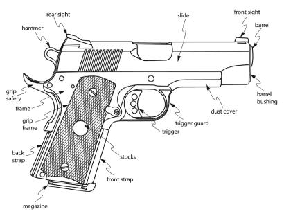
The major external parts of a semi-automatic handgun (also called a pistol).
