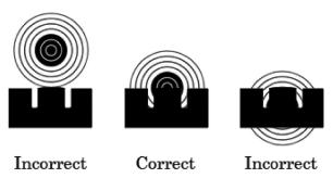
Incorrect and correct sight alignments for an open notch-and-post sight (typically used on handguns, but also available for rifles). The tops of the three posts should form a line through the point of aim. In the left image, the bullet will strike the target below the bullseye. In the center image, it will strike the bullseye. In the right image, it will strike above the bullseye.
