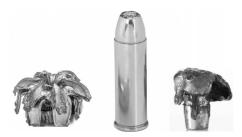
When bullets hit their targets, the soft lead deforms. The high-performance, expensive bullet on the left has "opened up" almost perfectly, whereas the one on the right has not.
