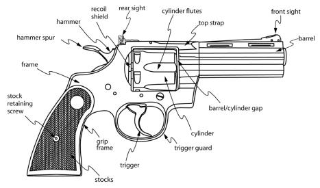
The major external parts of a revolver.
