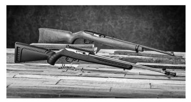
A pair of .22 caliber semi-automatic rifles. This is the same gun in two different configurations. The one in back has a traditional wood stock, while the one in front has a modern plastic polymer stock. The black gun also has a rail for mounting a riflescope, and it has a muzzle brake (mounted on the muzzle), which stabilizes barrel vibration so that the user more easily can stay on target for the second shot.
