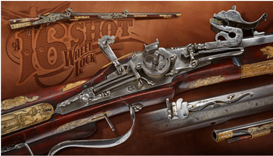
This German wheellock from the late sixteenth century fired 16 rounds with a single trigger pull. The ammunition is superposed—one round is stacked atop another.
