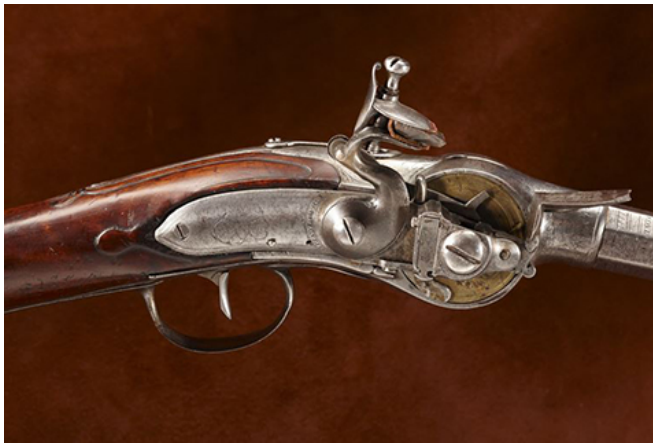
Cookson flintlock repeating rifle. The powder and ammunition magazines were in the buttstock; they were brought into the firing chamber by rotating the side lever.
