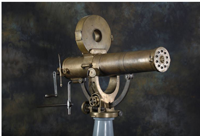
Gatling Gun , U.S. Navy Model. The blue-gray mount affixed the gun to a ship's deck. Land models of the Gatling Gun were mounted on portable tripods. Note the ten rotating barrels visible at the muzzle, and the hand crank at the rear. Because the Gatling is hand-cranked, it is a machine gun but not an automatic.
