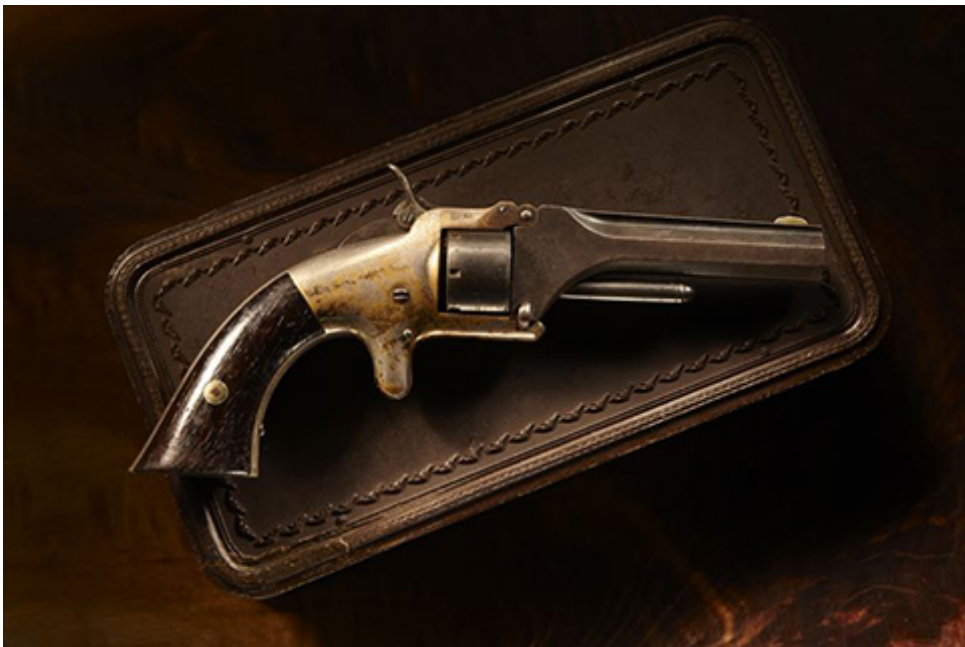
The Smith & Wesson Model 1 , the first U.S. firearm to use metallic cartridges. Manufactured 1857-60. The revolver rests atop its original case.
