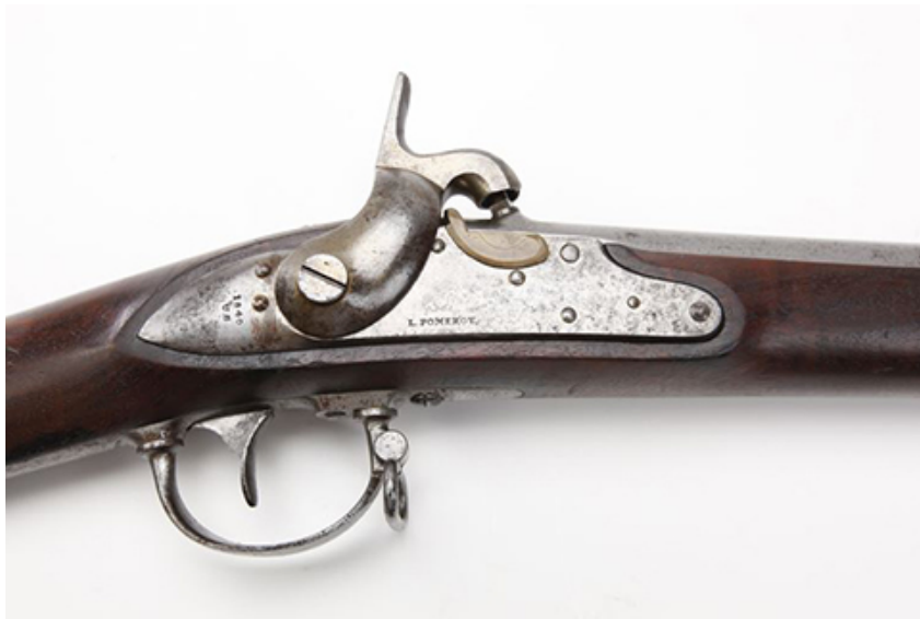
This Model 1816 flintlock musket was converted to percussion cap ignition.
